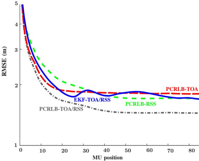
Fig. 3. Since the EKF is a suboptimal approach, this method does not reach the PCRLB obtained for TOA/RSS data fusion.
