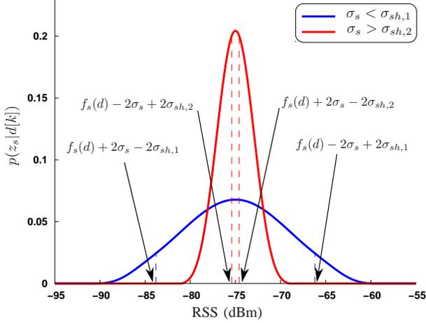
Fig. 1. The central piece of the RSS density varies depending on whether  $\sigma_s$  is greater or lower than  $\sigma_{sh}$ .
