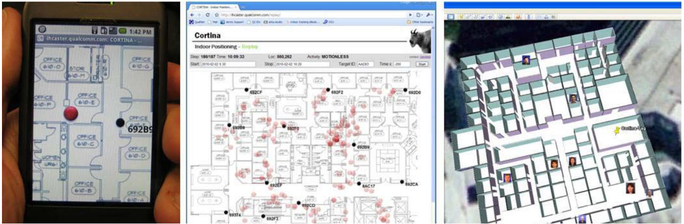
Fig. 6. left) AJAX web page that displays real-time information about the position of a target - the page can be accessed using a computer or a smart phone; center) web page that displays location traces over a period of time; right) Google Earth real-time visualization of the target's position.
