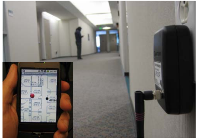
Fig. 1. On the right, one of the wall-plugged nodes of the Cortina positioning system. On the left, a web page that displays real-time position of the user.
