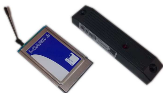
Figure 3. RFID interrogator and transponder used in the research ( i-Card III interrogator (left) and i-Q transponder (right) of the Identec Solutions long range active RFID system)
