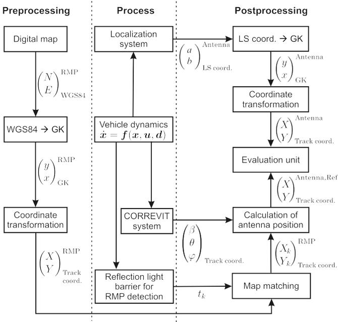
Fig. 2. Concept of the sensor data fusion
