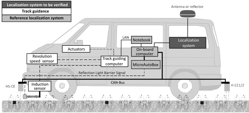
Fig. 1. Components of the reference measurement system
