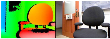
Fig. 8. View of the depth and RGB images from the robot Kinect® sensors.
