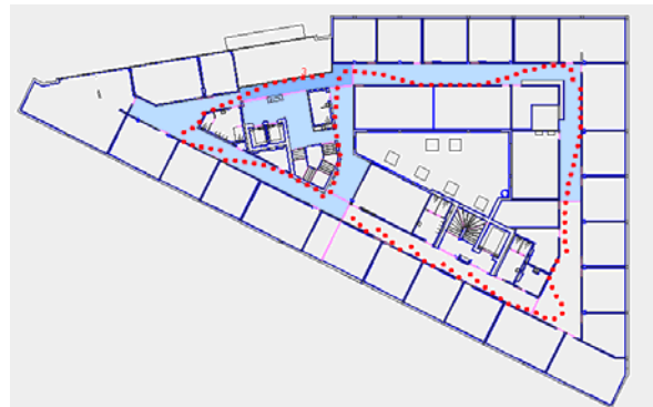
Figure 1. Map matching in a environment with disturbed earth's magnetic field caused by a railway track alongside the building
