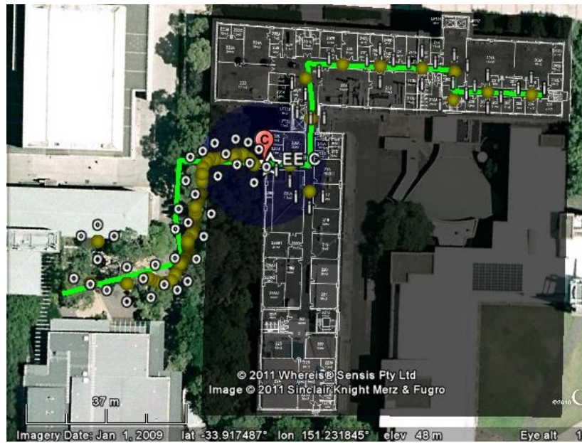
Figure 3. Transition from outdoor to indoor. The green line is the true path followed. The star symbol represents the position of the user when the software switched. Yellow dots with an “o” represent locations obtained with GPS, dots with an “i”, with Wi-Fi.
