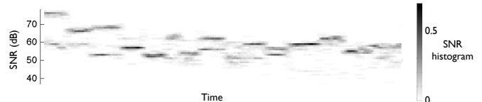
Fig. 1. Non-Gaussian Distributions of the Signal-to-Noise Ratio (SNR) of the RSSI. Data were recorded over 30min along a long corridor and for a single AP. The mobile would alternately stop for about two minutes at each location and move one meter further, repeating these steps for about 15 locations. The histograms have one bin per SNR level, and were constructed using 60s sliding windows and 10s steps.
