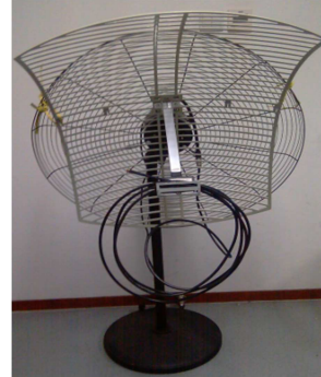
Fig.8. Rotating directional AP
