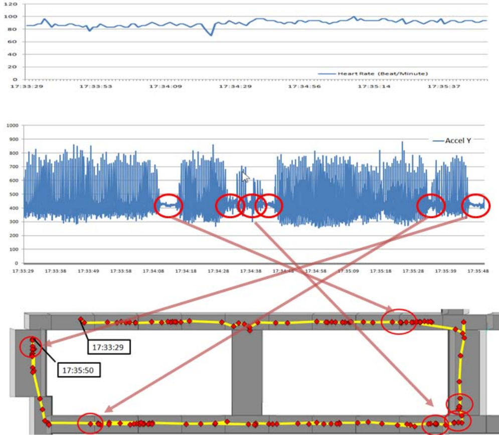
Fig. 6. An analytic result (user's heart rate (top), movement (middle), trajectory (bottom))
