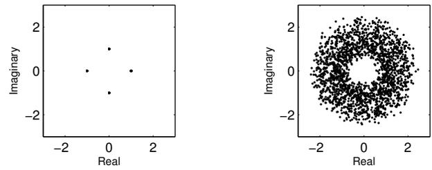
Fig. 8. Modulation constellation of the sent signal (left) and received signal (right).
