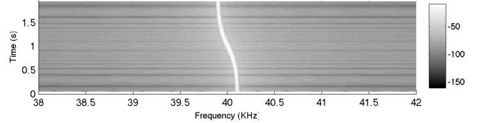
Fig. 3. Doppler effect into a 40 KHz sinusoid for a 1 m/s receiver speed.
