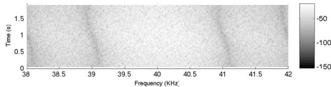
Fig. 7. Multiple reflections and Doppler effect into a communication signal modulated QPSK with a 40 KHz carrier for a 1 m/s receiver speed.
