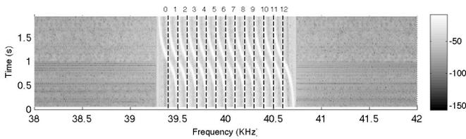
Fig. 6. Multiple reflections and Doppler effect into 13 carriers of a multi-carrier system operating from 38400 to 40600 for a 1 m/s receiver speed.
