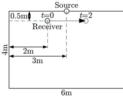
Fig. 2. Static source and receiver moving at 1 m/s in a 3 m high virtual room (Source and Receiver placed at 1 meter from the floor).
