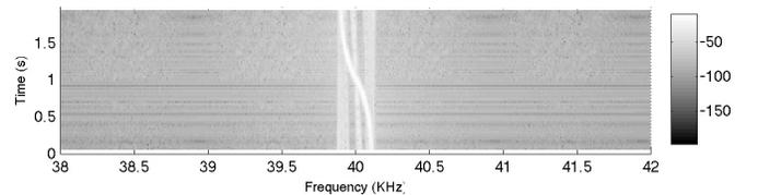
Fig. 4. Multiple reflections and Doppler effect into a 40 KHz sinusoid for a 1 m/s receiver speed.
