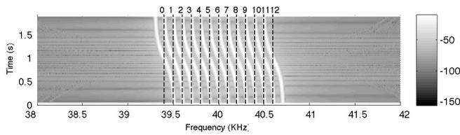
Fig. 5. Doppler effect into 13 carriers of a multi-carrier system operating from 38400 to 40600 for a 1 m/s receiver speed.
