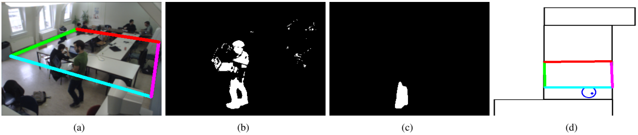
Fig. 1. The steps of the visual preprocessing. (a) the original image. (b) The foreground mask returned by the background subtraction. (c) Human filtering applied to the foreground mask. (d) The Gaussian kernel of the blob in image (c) mapped to the floor plan.
