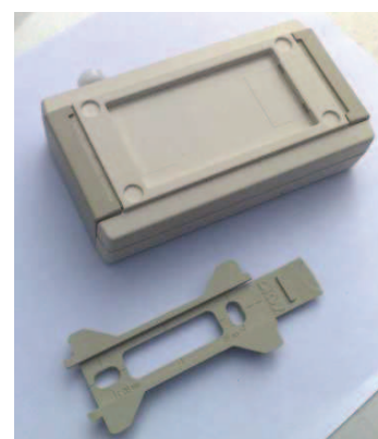
Fig. 2. The infrastructural node and its wall-mounting bracket.
