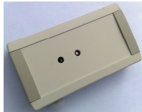
Fig. 1. The infrastructural “fixed” node showing holes for ambient-light, temperature/humidity sensors and movement sensor.
