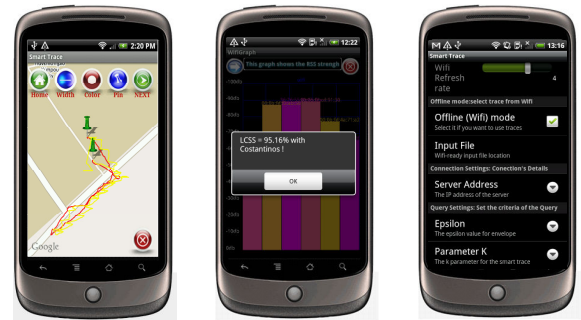
Fig. 2. Screenshots of the prototype system Left: The matched GPS trajectory displayed using Google Maps; Middle: A Query Response Message for RSS trajectories; Right: Parameter configuration and mode selection panel.
